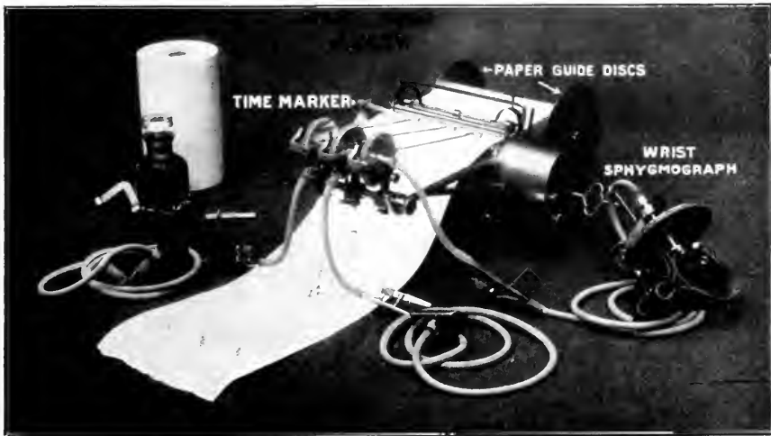
Fig. 2.—The Modified Mackenzie Ink Polygraph.
